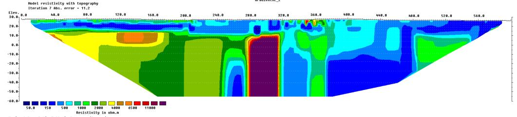
Horizontal scale is 7.66 pixels per unit spacing Vertical exaggeration in model section display = 1.15 First electrode is located at 0.0 m. Last electrode is located at 600.0 m. Unit Electrode Spacing = 2.50 m.
