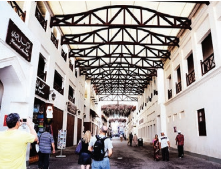
Soukh, Bahrain Manama: protection from the sun through a canvas above; reduces temperature at no energy cost. Picture: Internet
